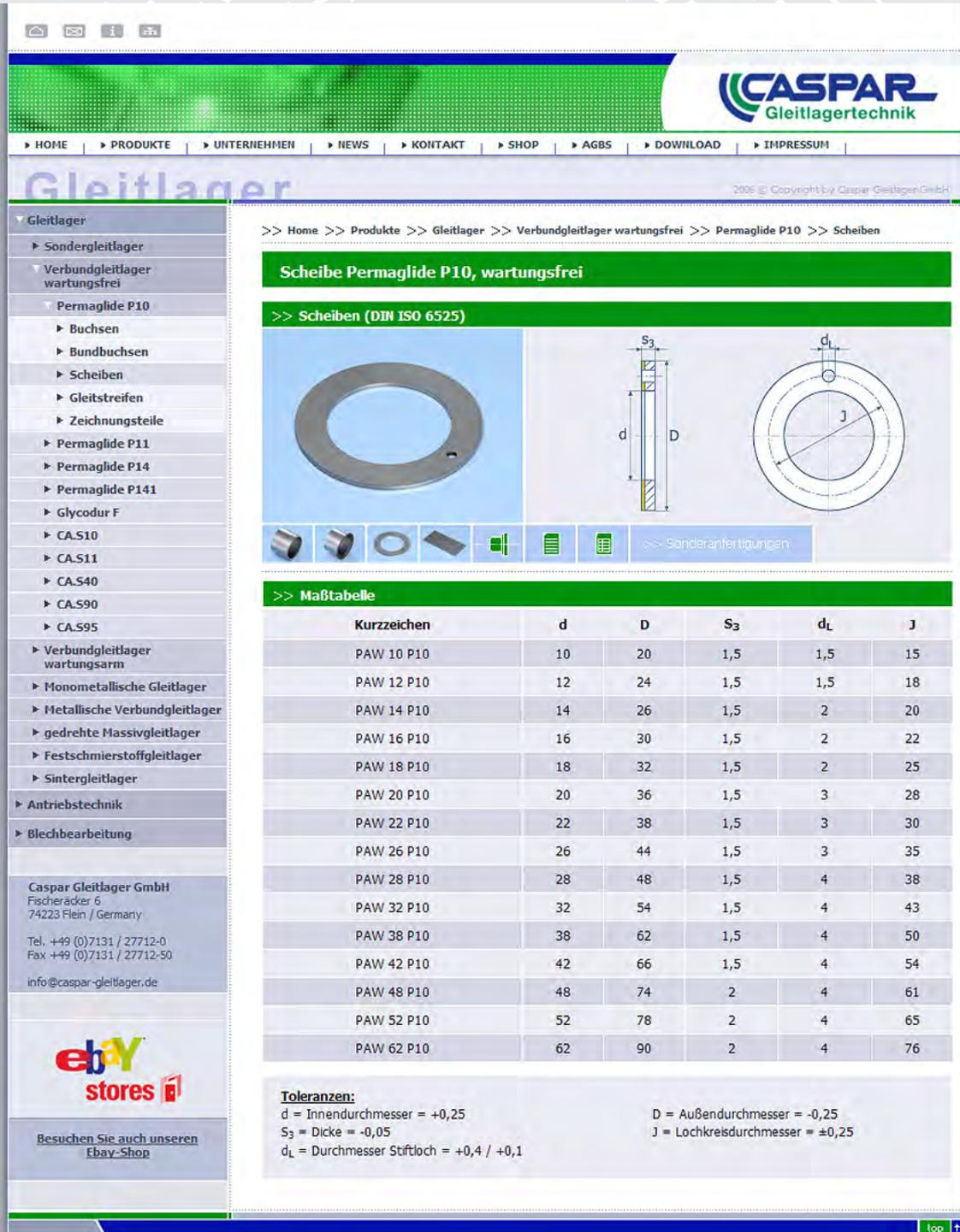
The screenshot shows the website for Caspar Gleitlagertechnik. The main content area displays the product 'Scheibe Permaglide P10, wartungsfrei'. It includes a 3D image of the ring, a technical drawing with dimensions  $d$ ,  $D$ ,  $S_3$ ,  $d_L$ , and  $J$ , and a table of dimensions for various sizes.
